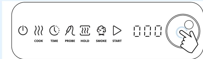
2. **Turn** the knob until the control displays "F or C".
