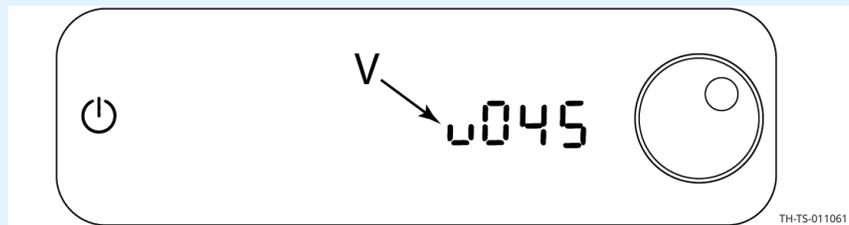
The control board (CB) software version displays.
