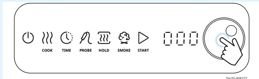
2. **Turn** the knob until the control displays "LOAD".
