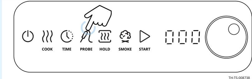
5. **Turn** the knob to set the probe alarm temperature.
