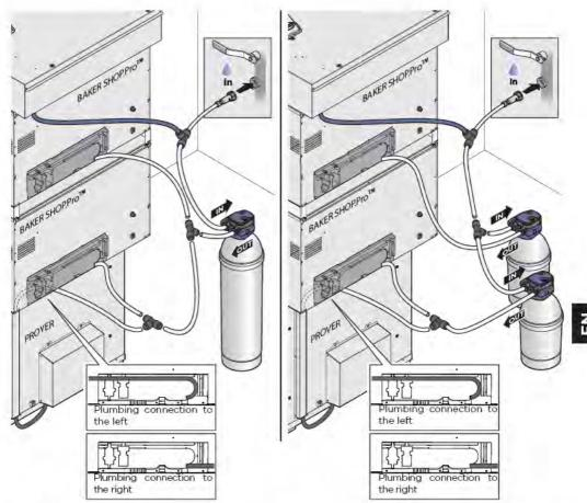
Should the water values for moisture generation differ from those shown, use a filter (UNOX.Pure/BAKERY.Pure).
